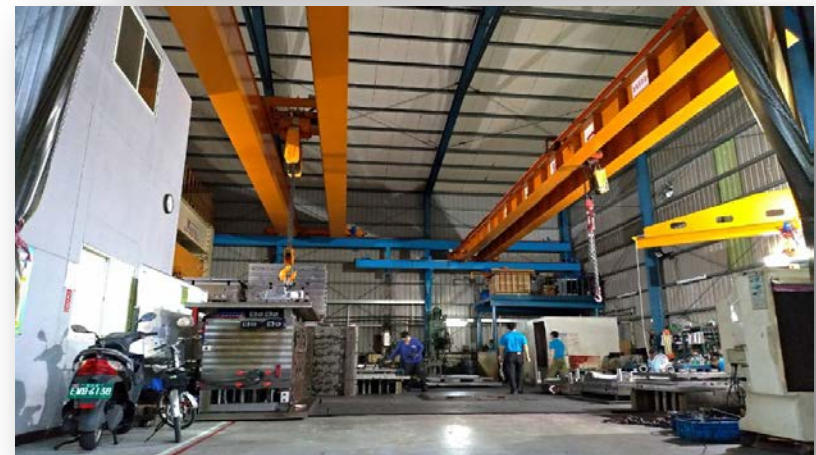
DOUBLE CRANE Lift max=28ton 15M X 12M X 4.5M
